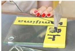
7) Once the colors are dry, remove the masking sticker and fix the characters by removing excess paint with a cotton swab or bamboo skewer knife.
