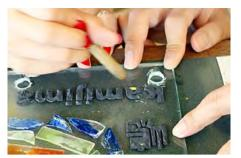
8) Complete by overlaying the nameplate on the painted background glass. Finish by placing the nameplate on the painted background glass. If the holes for the metal fittings are misaligned, the person in charge will correct them after completion.
