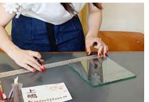
3) If you would like holes for metal fittings, there is a special machine you can use. Make 4 to 8 holes. Mark the place where you want to attach metal fittings with a marker. Make sure to mark 1.5cm to 2.0cm from the edge of the glass.
